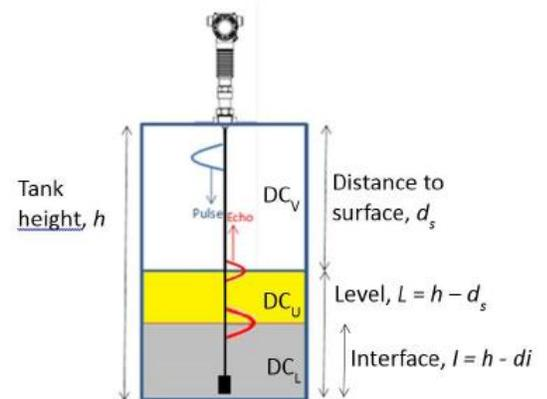
Figure 1:  $d_s$  = distance to surface;  $t$  = time for the pulse to travel distance  $d_s$ ;  $V_{wg}$  = speed of light in a vacuum on the probe;  $DC_v$  = dielectric constant of the material in the head space above the level (for air,  $DC_v = 1$ )
